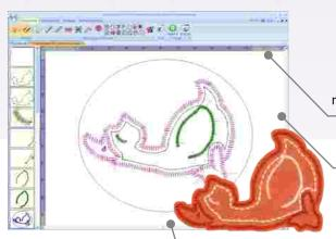
User friendly interface and complete control of the cutting / engraving parameters (power, cut speed, cut delay, repeat delay (to cool the fabric), fabric thickness, out of focus position)
